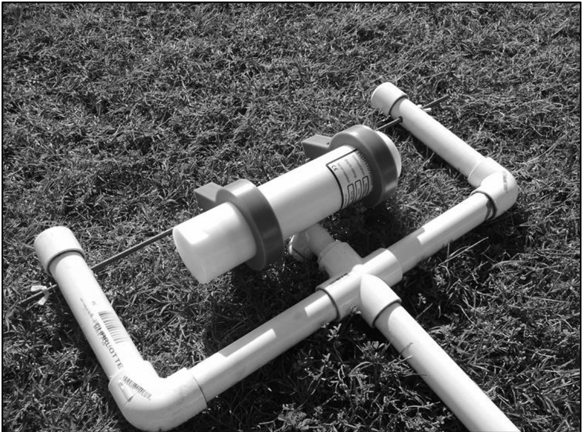
Figure A4. Mounts developed to hold sensors at deployment locations. Designed by Bret Webb.
