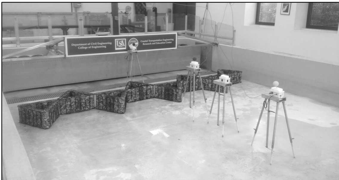
Figure 5. The University of South Alabama Wave Research Laboratory wave basin setup for conducting the experimental testing of the ReefBLK SM units.
